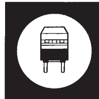
Stand-Off Lugs Minimize Solder-Creepage
